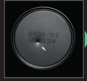
Characters and dents are recognized simultaneously using visible light.
