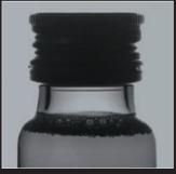
It is possible to recognize the state of the liquid due to IR transmission
