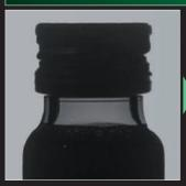
Transmission inspection is difficult for a brown vial using visible light
