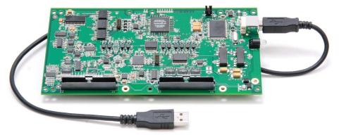
resolution. Four programmable gains (1, 2, 4, and 8) are provided to support input signal ranges of  $\pm 10$  V,  $\pm 5$  V,  $\pm 2.5$  V, and  $\pm 1.25$  V for each individual channel.
