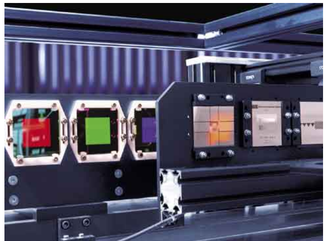
The Basler eXcite is measured by the CTT+ according to the EMVA 1288 standard
