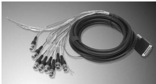
Connect the cable's DVI connector to one of the DVI connectors on Matrox Helios XA. Then, connect the BNC connectors as follows.
