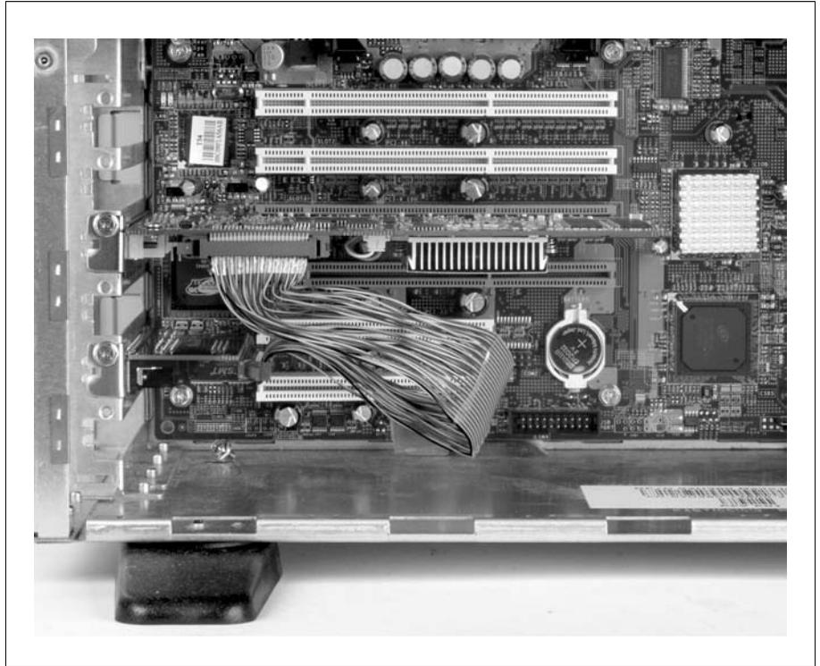
6. Anchor the adapter board's bracket to the chassis using the screw that you removed in the previous section.
